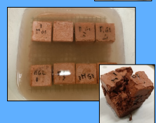
Salt crystallization test (UNI EN 12370:2020)
